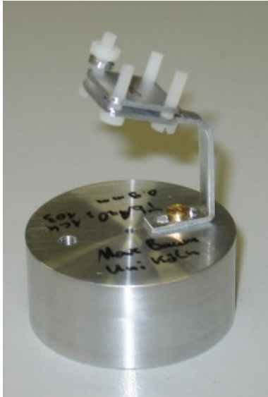
Figure 6.3: Sample holder of TbMnO_3 . The electric field is applied by two aluminium plates which are fixed by four nylon screws. The sample is 0.9 mm thick.
