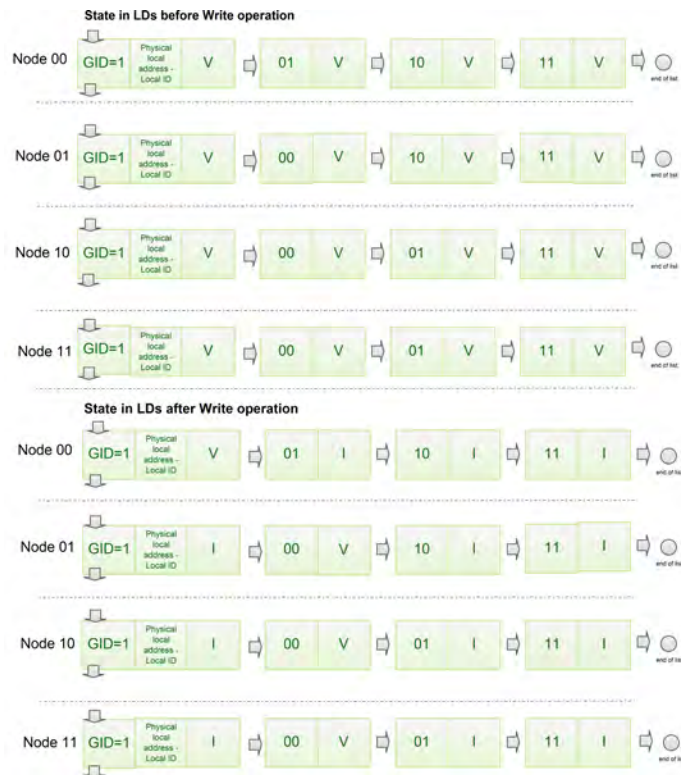
Figure 3.16: LDs' pre and post states for Scenario 3, assuming that GlobalID of shared block is 1
