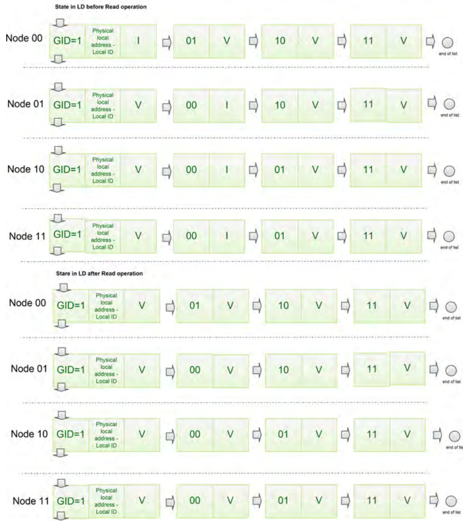
Figure 3.14: LD's pre and post states for Scenario 2, assuming that GlobalID of shared block is 1
