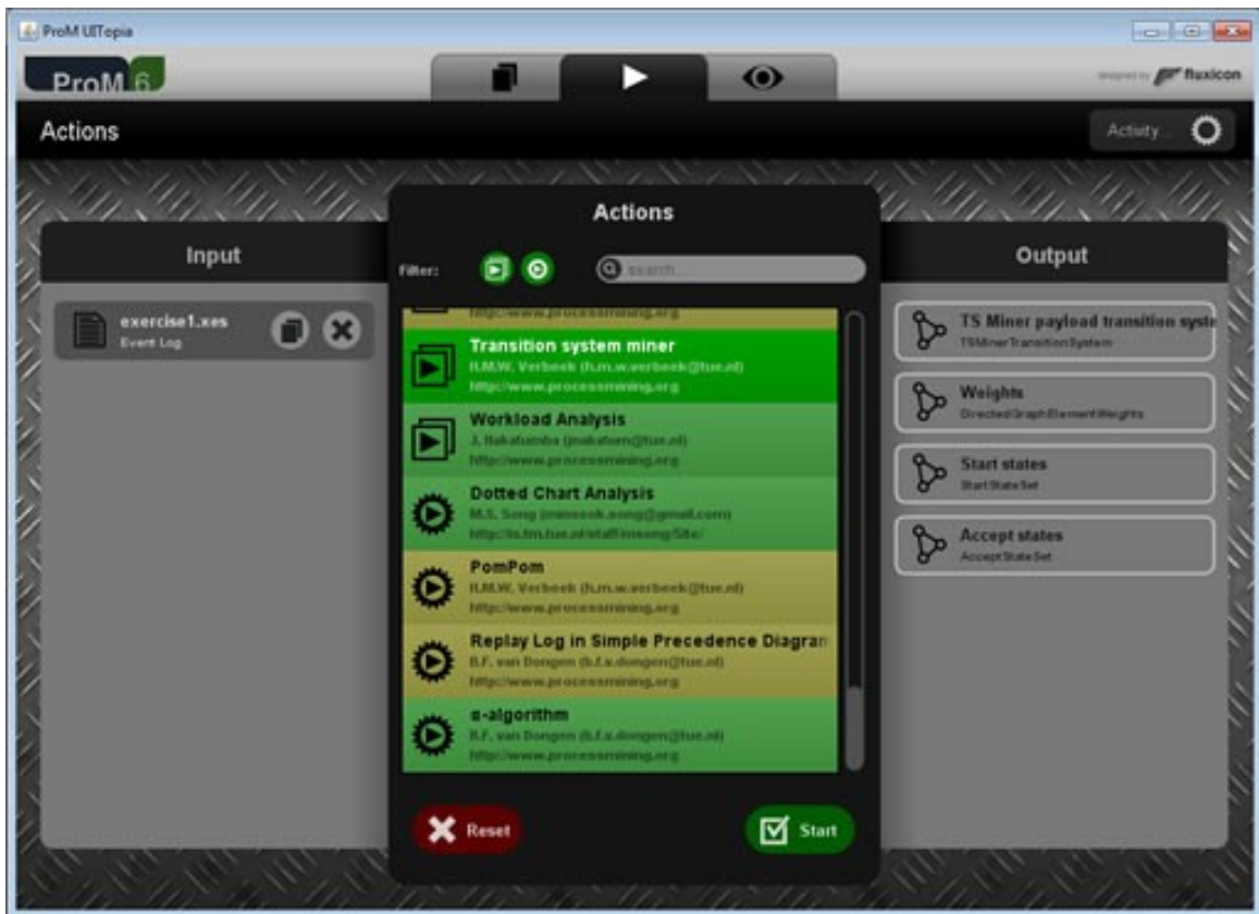
Illustration 8: ProM screenshot from official website with possible actions in the center (Transition system miner is selected), inputs, required for the selected action on the left (an event log is needed) and outputs, produced by the selected action on the right (payload transition system, weights etc).
