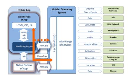
Figure 2.8: Architecture of Hybrid Mobile Application Using PhoneGap Framework (13)
