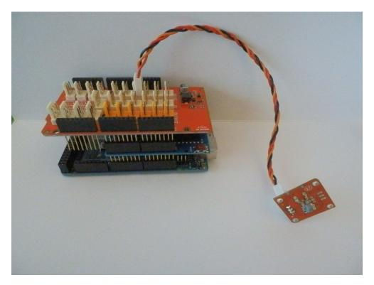
Figure 4.2: From Bottom: Arduino Mega ADK, Wireless Shield, Sensor Shield and Temperature Sensor.
