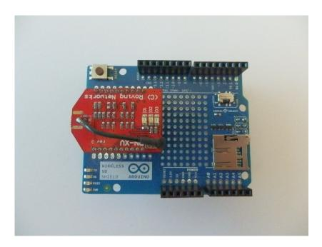
Figure 2.11: Arduino Wireless Shield
