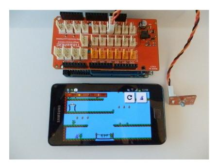
Figure 5.3: The Game Setup: Arduino Mega ADK with Extended Shields and Samsung Galaxy S2
