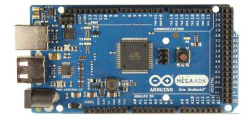
Figure 2.10: Arduino Mega ADK (1)
