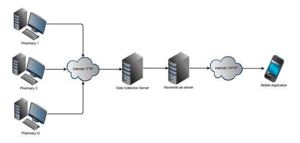
Figure 3.1: An overall diagram of how data flows from pharmacy to mobile application.
