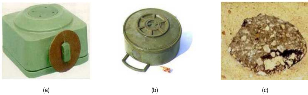
Figure 5.6. (a) Box like plastic landmine, (b) AP mine having a shape of cylinder and (c) Irregular rock clutter.
