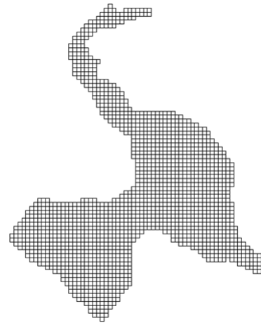
(b) A set of initial staircase mesh
