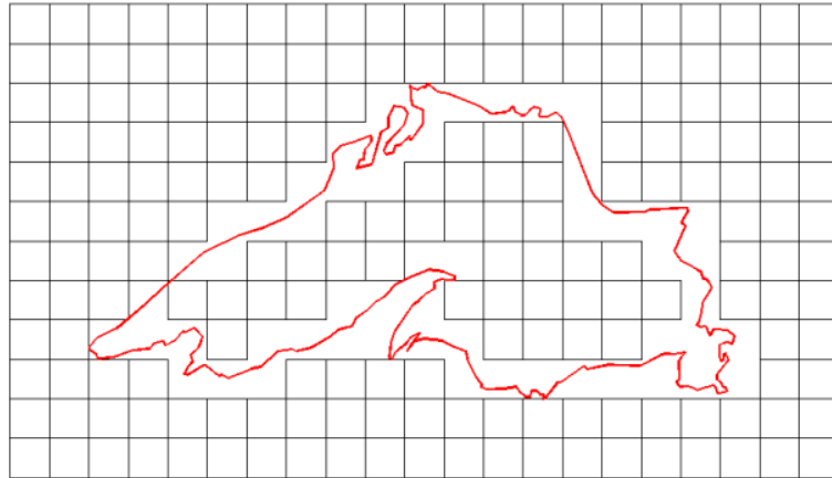
(a) Elements inside and outside the boundary are selected from a Cartesian mesh.
