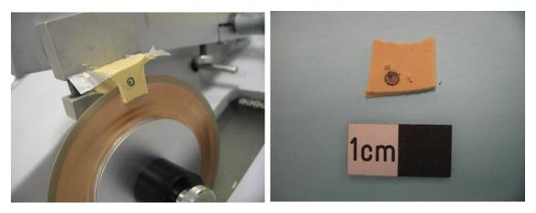
Figure 3 plaster block and root positioned to allow cutting of consecutive measured sections
