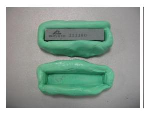
Figure 1 creating a mould using dental impression material
