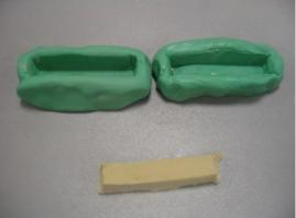
Figure 2 plaster block removed from mould
