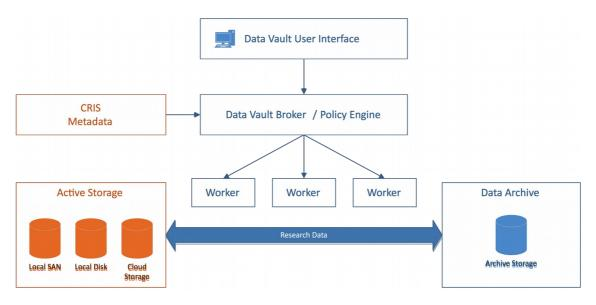
Figure 2. System architecture of the DataVault.
