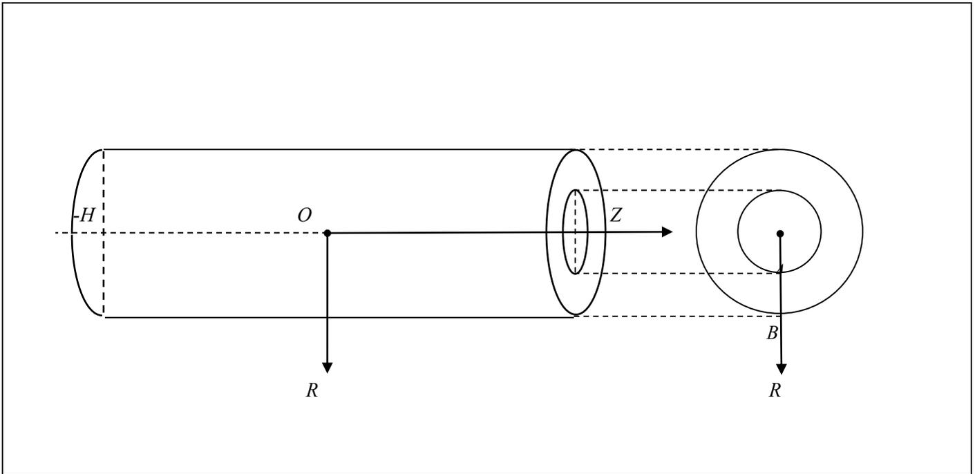
FIGURE 1: Nomenclature of a finite hollow circular cylindrical tube and its cross-section in the reference configuration. Nomenclature in the current configurations is obtained by replacing capital letters with their low case version.
