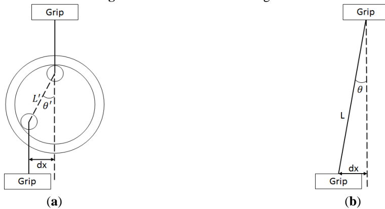
Figure 9. (a) Misalignment of small ring specimen when pins are not in line; (b) Misalignment of a standard specimen.
