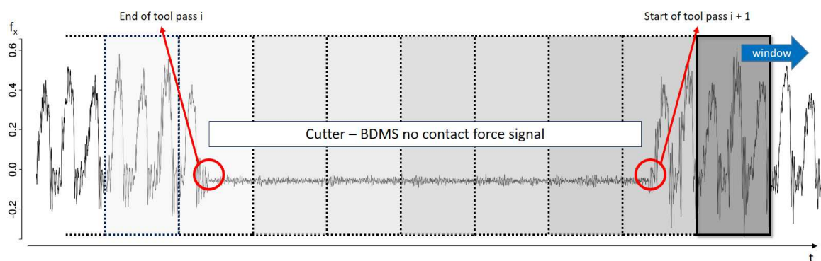
Figure 5. Detection for the removal of the no contact force signal between the cutter and the bright drawn mild steel (BDMS) workpiece. A fixed size window moves along the acquired signal searching for the start and end of a small subsequence of very small values denoting the end of tool pass i and start of tool pass i + 1 .
