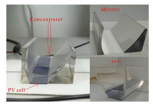
Fig. 8. The prototype of proposed CPV module.
