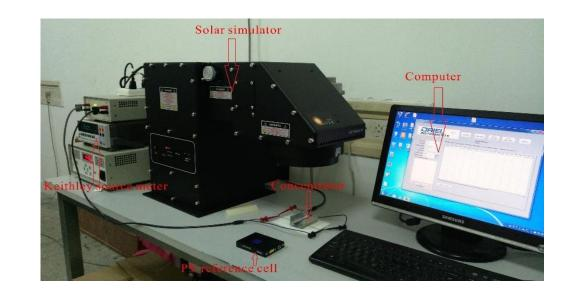
Fig. 9. The experiment setup.
