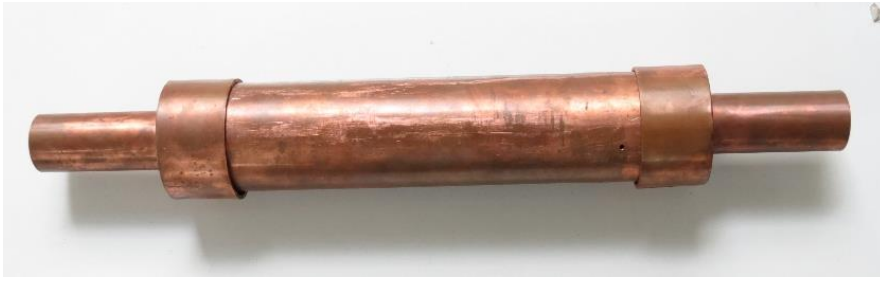
Figure 2a. Copper Packed Bed Vessel with Inlet and Outlet Caps
