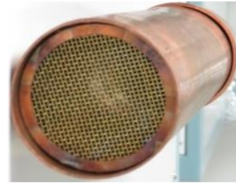
Figure 2b. Packed Bed Showing Mesh Insert
