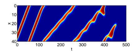
Figure 13: A subcritical Hopf bifurcation of a moving pulse. At t = 100, h is switched from 0.05 to 0.07.  $u_e$  is plotted, red high and blue low. Periodic boundary conditions are used. Other parameters are as in Fig. 12.
