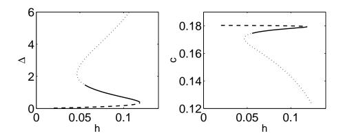
Figure 16: Width (left panel) and speed (right panel) of a travelling pulse as a function of h, with inverted Mexican hat connectivity. Solid lines represent stable one-bump solutions and dashed unstable, while the dotted lines indicate a solution of (41)-(42) which is not a one-bump solution. Parameters are  $v_e = 0.2, v_i = 1, \alpha_e = 1, \alpha_i = 1, \Gamma = 0.7, \sigma_e = 2, \sigma_i = 1$ .
