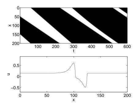
Figure 15: A wide moving pulse for which the back travels slower than the front, leading to the formation of an "anti-pulse". Top:  $u_e$  is plotted, with black being high and white low. Bottom:  $u = u_e - u_i$  once the anti-pulse has formed. h = 0.05, so most of the domain is active. Other parameters are as in Fig. 9.
