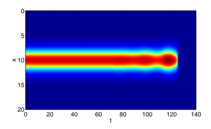
Figure 5: Instability of a stationary bump due to a subcritical Hopf bifurcation. At t=70 we switched  $v_i$  from 1 to 0.2 (and a small random perturbation was added). Other parameters are  $v_e=1, \alpha_i=\alpha_e=1, h=0.1, \sigma_e=1, \sigma_i=2$  and  $\Gamma=1$ .  $u_e$  is plotted, with red high and blue low. 200 spatial points were used.
