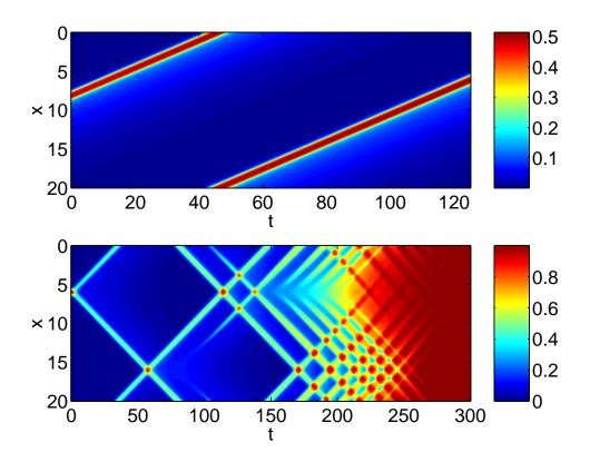
Figure 17: Top: a stable travelling pulse for inverted Mexican hat connectivity. Bottom: the interaction of two such travelling pulses leads to complex behavior.  $u_e$  is plotted. Note the different time scales. Parameters are  $v_e = 0.2, v_i = 1, \alpha_e = 1, \alpha_i = 1, \Gamma = 0.7, \sigma_e = 2, \sigma_i = 1, h = 0.07$ .
