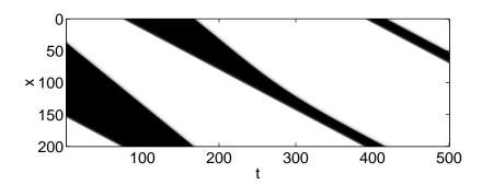
Figure 14: A wide moving pulse for which the back travels faster than the front. The eventual solution is a moving pulse, of the type analysed in Sec. 4.2.  $u_e$  is plotted, with black being high and white low. Periodic boundary conditions are used. h = 0.115 and other parameters are as in Fig. 9.
