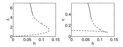
Figure 12: Width ( $\Delta$ , left panel) and speed (c, right panel) of a moving pulse as function of h. A solid line indicates stability, while a dashed one indicates instability. There is a Hopf bifurcation on the top branch. Other parameters are  $\Gamma=1, \sigma_e=1, \sigma_i=2, \alpha_e=1, \alpha_i=0.3, v_e=v_i=1$ .
