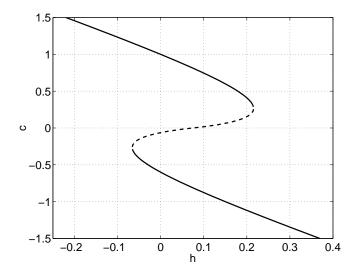
Figure 9: Front speed as a function of h. Stable fronts are represented by solid lines, unstable by dashed. Parameters are  $\Gamma=0.85, \alpha_e=1, \alpha_i=0.1, v_e=v_i=1, \sigma_i=2$  and  $\sigma_e=1$ .
