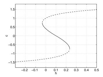
Figure 10: Front speed as a function of h. Parameters are  $\alpha_i = \alpha_e = 1, v_e = v_i = 1, \sigma_e = 1, \sigma_i = 2, \Gamma = 0.8$ . The solid branch is stable, while the dashed ones are unstable.
