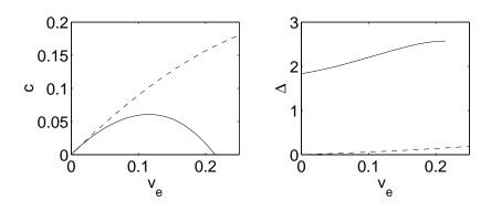
Figure 11: Left: pulse speeds as a function of  $v_e$ . Right: pulse widths as a function of  $v_e$ . Solid lines indicate stable solutions, dashed unstable. Note that the speeds are always less than  $v_e$ . Other parameters are  $\alpha_i = \alpha_e = 1, v_i = 1, \sigma_e = 1, \sigma_i = 2, h = 0.1, \Gamma = 1$ .
