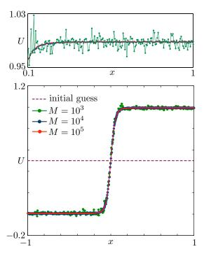
Fig. 5.4: Macroscopic fronts computed with the Newton-GMRES solver (see also Figures 5.5(c) and 5.5(d)). The initial guess for all cases is a mixed state  $U(x) \equiv 0.5$ . The inset on top shows that the noise in the macroscopic profile is controlled by increasing the number of realizations.
