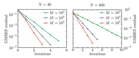
Fig. 5.3: Convergence of GMRES iterations for the problem DF(U)V = -F(U), where U is a macroscopic front and  $DF(U) = I - D\Phi_T^M(U)$ , for different numbers of agents N and numbers of realizations M. Jacobian actions are computed with weighted lifting and  $\varepsilon = 10^{-5}$ .
