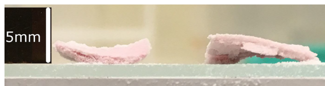
Fig. 6. Warping of 3D printed 9:1 cellulose LBG powder.
