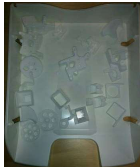
5c: An FDM extruder kit with 26 components
