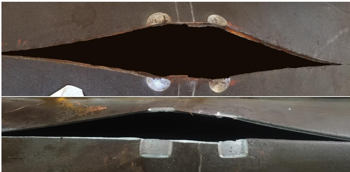
Figure 11: Typical failure of circular and curved boxed defects spaced by a distance of 6t in the X52 pipe
