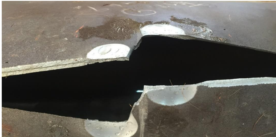
Figure 12: Failure behaviour of diagonal circular defects spaced by a distance of 0.5t in the X52 pipe
