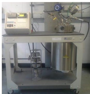
Figure 4. Modified SATS test set-up consisting of pressure vessel, pressure and temperature controllers, and bitumen sample holder for producing CO 2 -modified bitumen.
