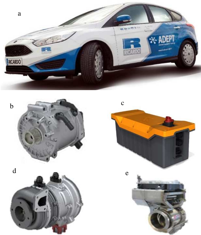
Figure 6. The ADEPT demonstrator vehicle (a), fitted with the 48V mild hybrid system, including B-ISG (b), 48V UltraBattery (c), TIGERS e-Turbine (d), and Exhaust Control Valves (e)
