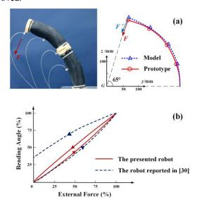
Fig. 10. (a) Bending deformation due to an external force, (b) Bending-return characteristics of the robot
