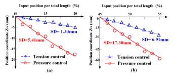
Fig. 11. Relationship between the inputs of the TEPM  $A_{1,3}$  and the position coordinate  $z_{\rm ed}$
