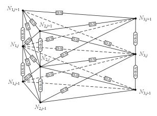
Fig. 4. Two segments represented by the mass-damper-spring systems  $(N_{ij}, i=1,2,3,\ j=1,...n-1)$
