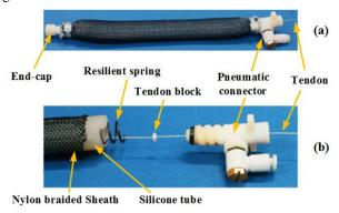
Fig. 3. TEPM Configuration (a) Overview of a TEPM (b) Exploded view of the TEPM  $\,$
