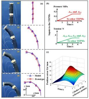
Fig. 9. Whole arm bending dynamics
