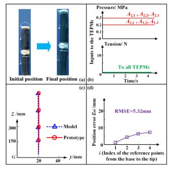
Fig. 7. Elongation of the robotic prototype
