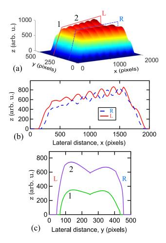
**Fig. 5** (Color online) (a) Surface plot of simulated nanotrack morphology employing the model described in text. The two axial lines along the simulated nanotrack (one solid red and the other broken blue) indicate the paths of the line height scan data presented in (b), and (c) shows two cross sectional height scans obtained from the locations indicated in (a). The horizontal axes here are given in pixels.
