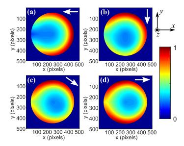
**Fig. 4** (Color online) Normalized nucleation (in the *z*-direction) rate determined by the model at the liquid-solid interface A for differing  $\alpha$  values of (a)  $0^{\circ}$ , (b)  $90^{\circ}$ , (c)  $145^{\circ}$ , and (d)  $180^{\circ}$ . The depicted coordinate system relates to the axes shown in Fig. 3 and the white arrows indicate the relative flux directions for each angle.
