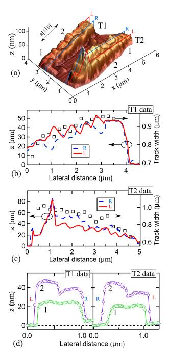
**Fig. 2** (a) AFM micrograph of two antiparallel nanotracks, labeled T1 and T2. The two axial lines along both nanotracks (one solid red and the other broken blue) indicate the paths of the line height scans presented in (b) and (c). The nanotrack width data in (b) and (c) were determined via multiple line height scans measured orthogonally to  $\pm [1\bar{1}0]$ , and (d) shows two of these scans obtained for both nanotracks at the locations indicated in (a).
