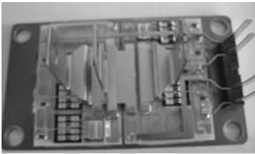
Fig.1. Example of a typical (dual switch) half bridge IGBT power module (300A,1200V) consisting of two IGBTs and two Diodes
