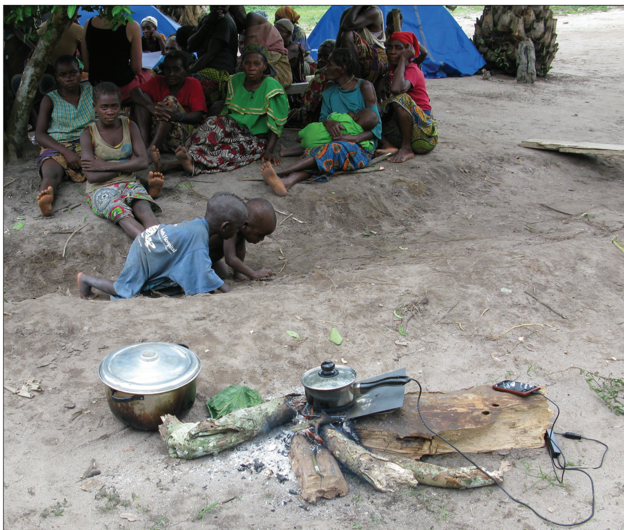
Figure 4 Charging a smartphone with the Hatsuden Nabe HC-5
