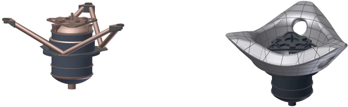
Figure 3 - Different support structure concepts considered during the drive to lose weight. left : a carbon fiber replacement using struts. right : a solid molded carbon shell structure mount.
