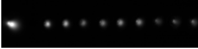
Figure 6. Illuminated fibers (740 nm source, 5 ms exposure) through slit forming optics. The simultaneous reference fiber is on the left, with the nine science fibers following after a single fiber gap.
