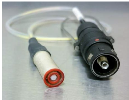
Figure 7. A Starbug for TAIPAN. The left element (white/red) is the Starbug with a science fiber in the center and three metrology fibers in the gap between the two (red) piezo sleeves. The connector on the right mates to a science fiber feeding the spectrograph, the three metrology fibers that are back-lit by LEDs, and power to drive the piezos.
