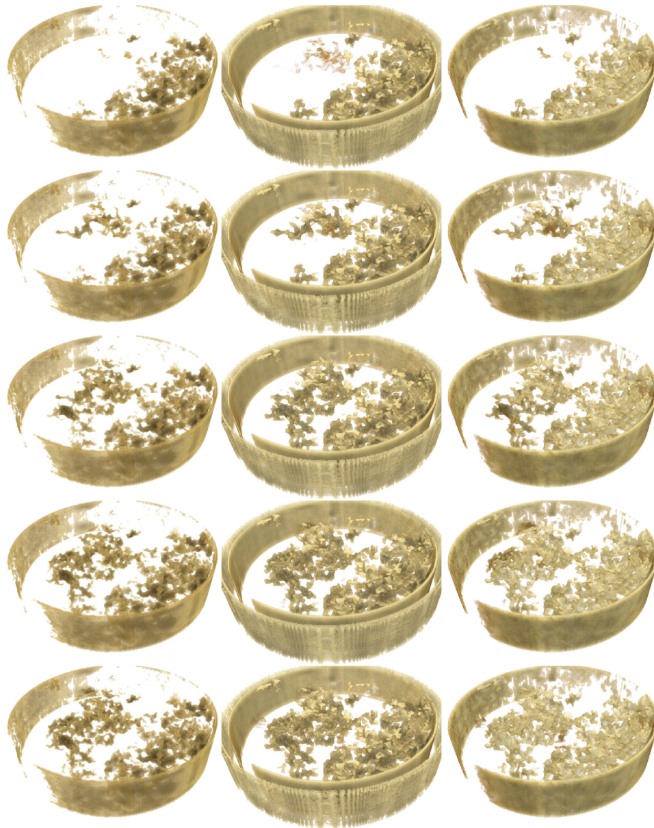
Fig. 1. 3D renderings of five sequential volume frames (proceeding top-to-bottom). Each frame is calculated as a difference image between the initial and current reconstructed states of the sample [i.e. \mu(\mathbf{x}, t) ]; in a drainage experiment this difference is primarily due to air infiltrating the pore space. The middle column shows the results of the reference FBP reconstruction ( Visualization 1 ). The left column shows the reconstruction produced by our empirical SIRT-based algorithm [4]. The right column shows reconstructions performed using Eq. (5) ( Visualization 2 ).
