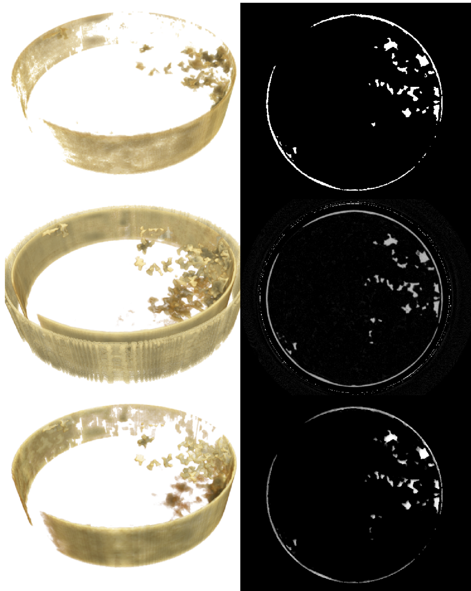
Fig. 2. Reconstructed 2D (right) and 3D (left) slices through a Bentheimer sandstone during drainage, calculated as a difference image between the initial and current reconstructed states of the sample [i.e. \mu(\mathbf{x},t) ]. 2D slices are a 480 \times 400 pixels ( 6.7 \times 5.6 mm), taken normal to the rotation axis. Middle row : a reference reconstruction from full data, using FBP. In the upper right is a pore which displays partial volume effects. This violates our assumption that the rock is present at only a single grey level. Top row : reconstruction from every 10th viewing angle, using an empirical SIRT-based 2-phase flow algorithm [4]. Bottom row : reconstruction from every 10th viewing angle, using MLTR-like algorithm [Eq. (5)]. Note successful reconstruction of partial volume effects.
