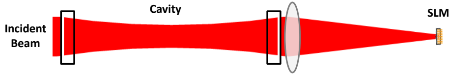
Figure 7.1: A Kahlili cavity. Using an SLM as the third mirror in a Kahlili cavity can reduce the transmitted field to zero and ensure all the light is reflected back into the interferometer even if the quality of the second mirror is poor.
