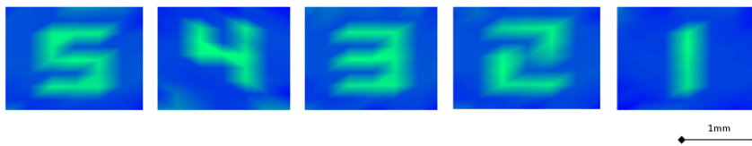
Figure 5.20: Demonstration of higher-order spatial phase manipulation. The blue rectangle shows the individual phases across a 9 by 7 matrix of elements each of which has been spatially tagged with an orthogonal code. The numbers are created by adding a fixed offset to the code modulation on some of the segments of the SLM.
