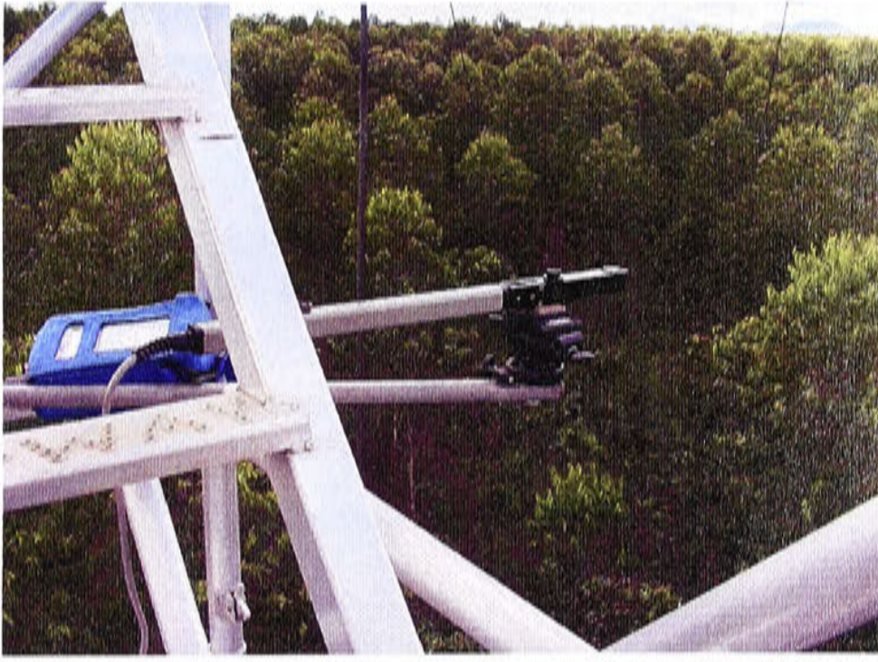
a) Sensor of plant canopy analyser LAI-2000 above the canopy
