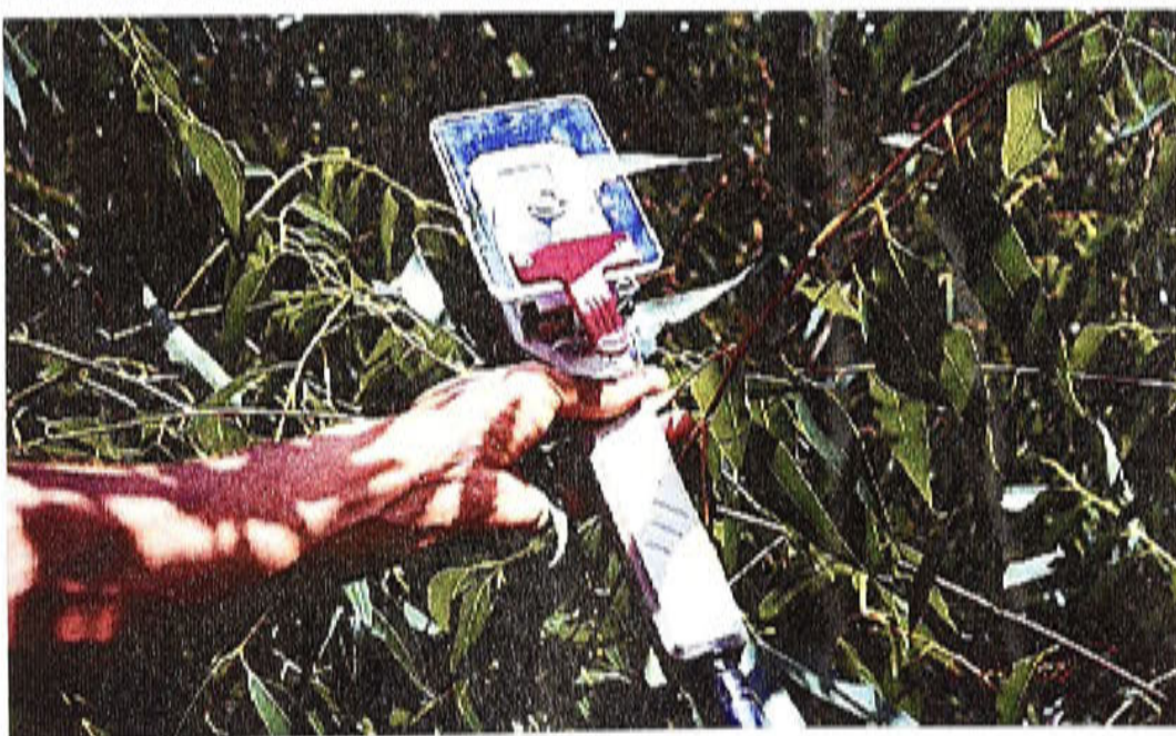
c) Measurement of stomatal conductance
