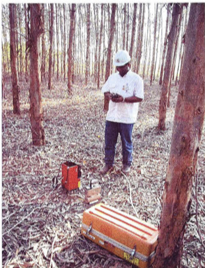
a) Measurement of soil moisture using neutron probe
