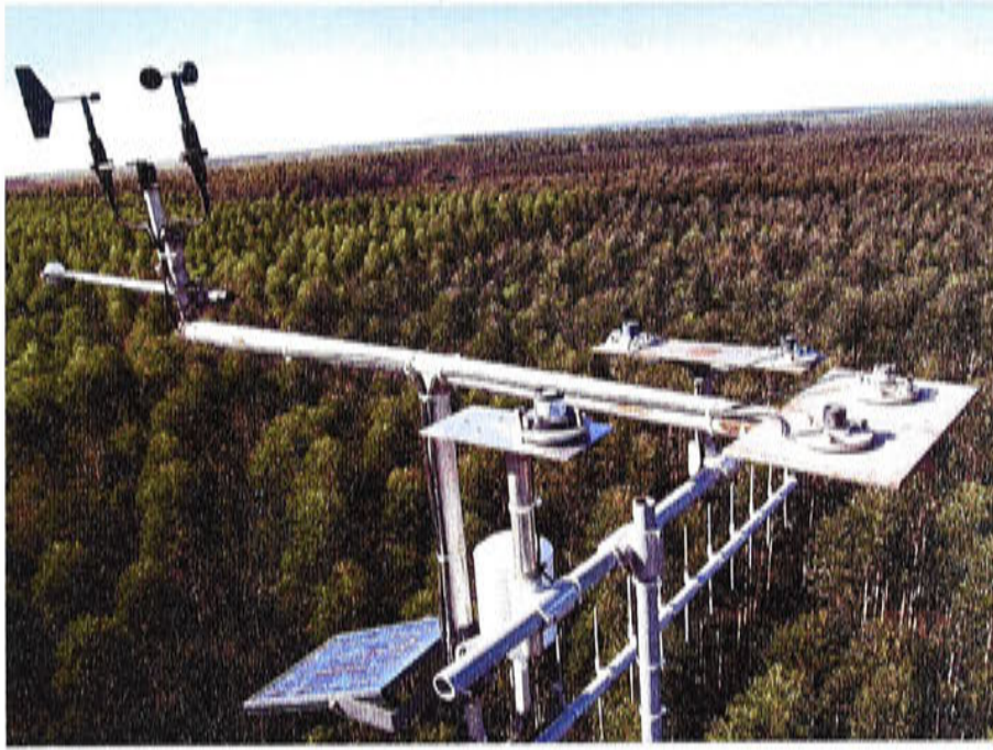
a) Microbacia weather station - sensors of wind direction and speed, net radiation, PAR, global radiation temperature and relative humidity, solar panel and antenna for data transmission
