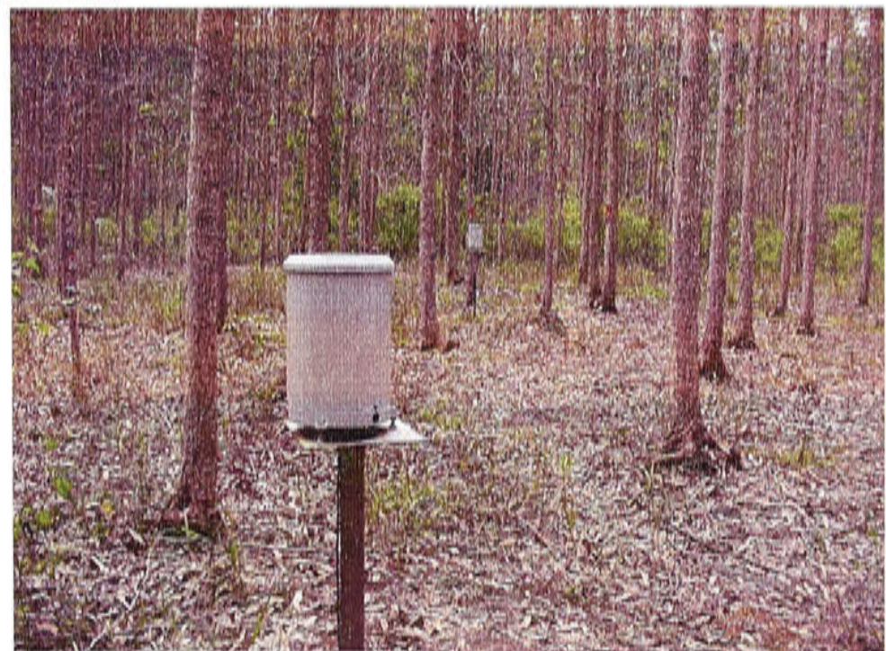
d) Raingauges below the tree canopy to measure rainfall interception
