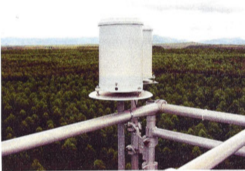
c) Raingauges above the tree canopy
