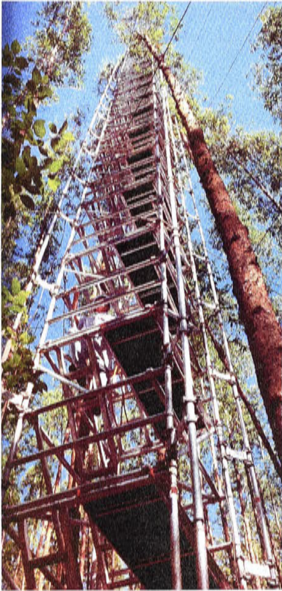
a) Tower used for ecophysiological and meteorological measurements
