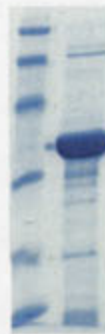
Figure 3.14: Purity of syringe purified MPH with purification workflow IV after concentration. Molecular weights of proteins in molecular marker, from top to bottom are 97.4, 66.2, 45.0, 31.0, 21.5, 14.4 kDa.
