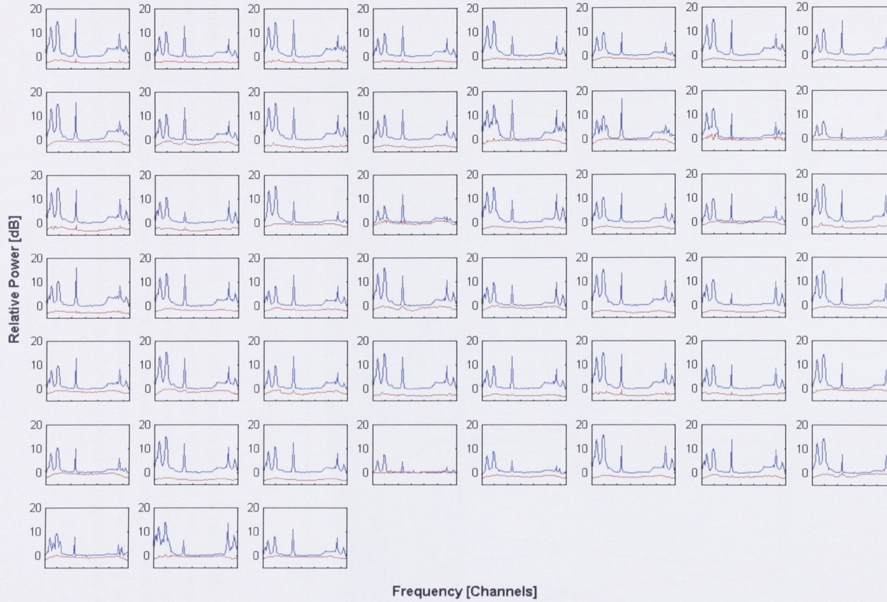
Figure 5.8 MWA Solar total power spectra at 261.12 MHz. Relative power [dB] is plotted as a function of frequency channel 1-128. The channel spacing is 10 kHz and the integration time one second. Blue: Original spectra. Red: Corrected spectra (first five eigenvalues replaced with a noise estimate). The effectiveness of the cancellation on only some channels raises interesting questions. In particular note the similar nature of the interference in feeds one and nine, and the way in which feed nine cancels more effectively.
