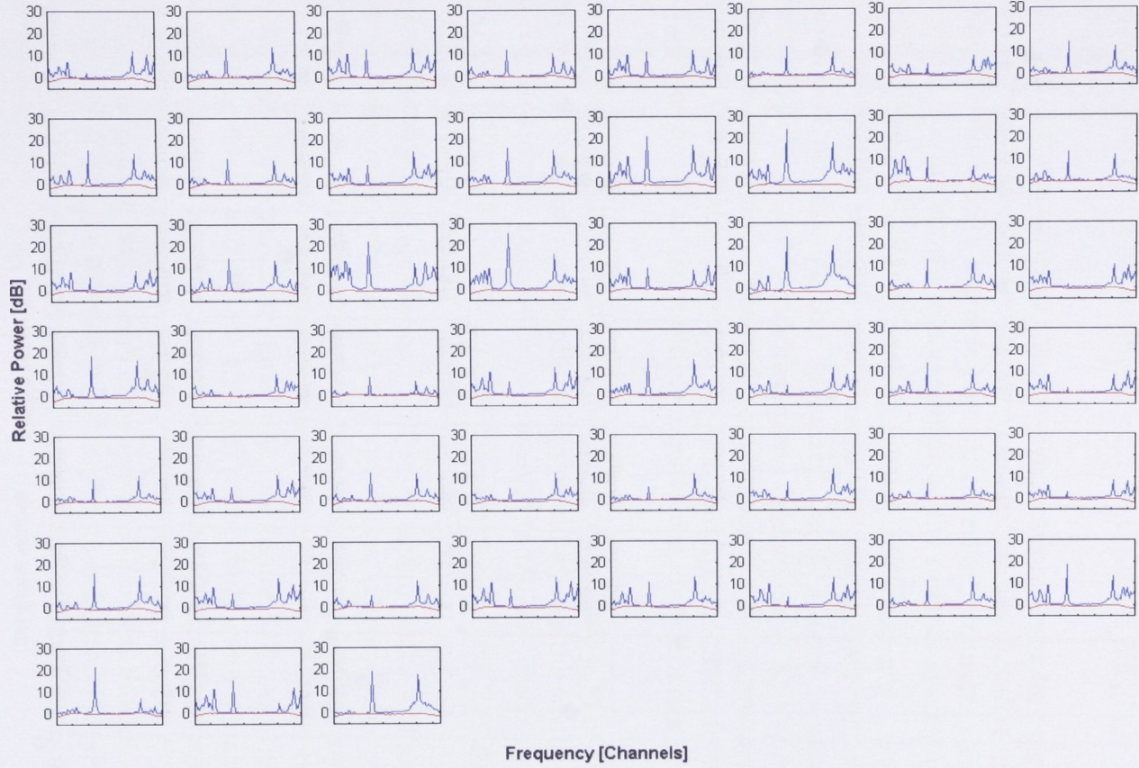
Figure 5.4 MWA Hydra A total power spectra at 261.12 MHz, correction comparison after replacing the first 8 eigenvalues with a noise estimate. Channel spacing is 10 kHz and the integration time one second. Blue: The original spectra. Red: The corrected spectra.
