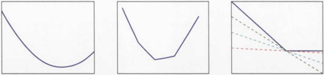
Figure 1.2: Left: the objective function of a typical regularized risk minimization problem (plotted along a direction) is convex, but zooming into the region around the optimum (center) reveals its nonsmooth points. Right: the hinge loss: l(f) := \max(0, 1 - f) (solid line) is nonsmooth; the slope of any line that is tangential to l at a point (e.g., dashed lines) is a subgradient.
