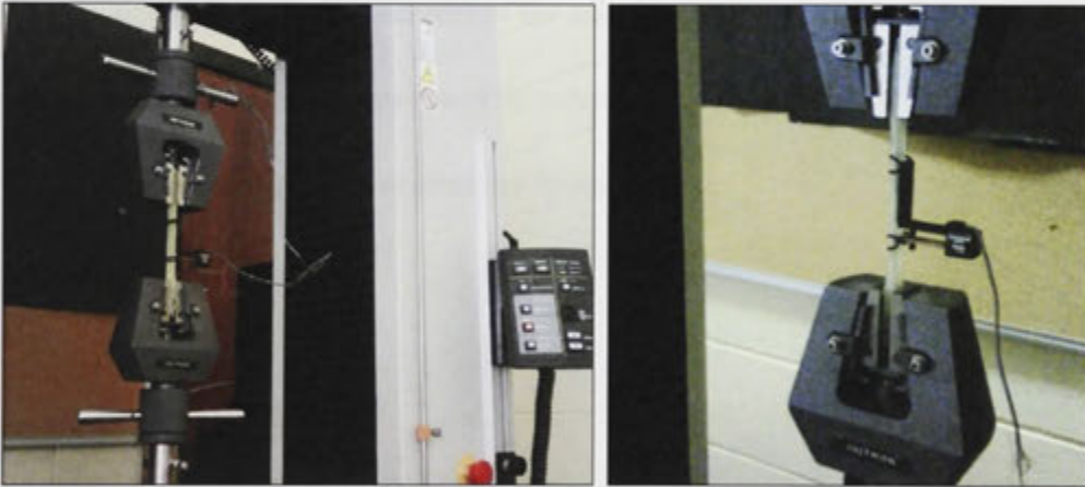
Figure 4.16: Instron machine and tensile testing set-up.
