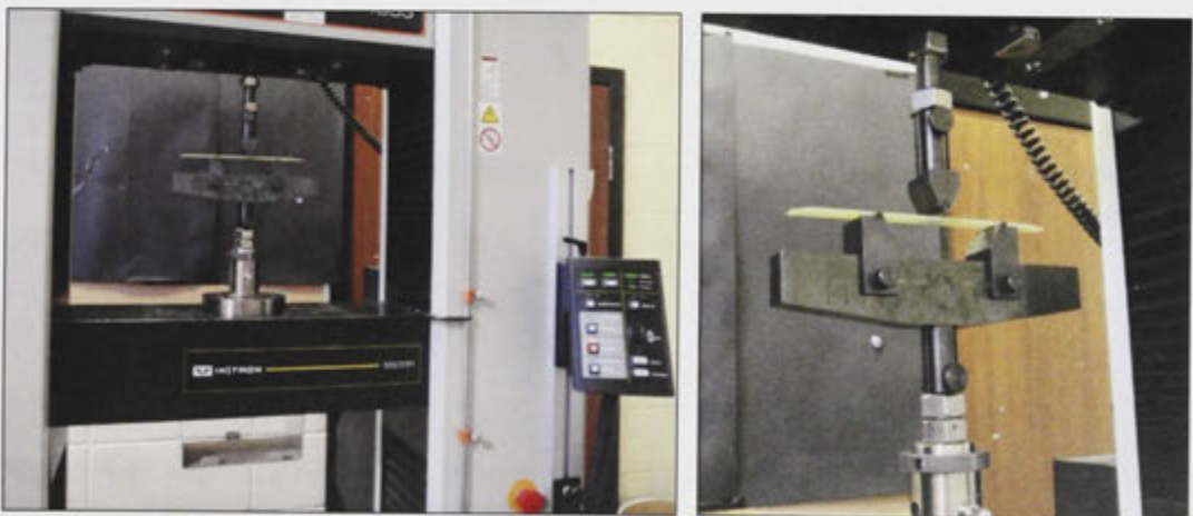
Figure 4.18: Instron machine and flexural test.
