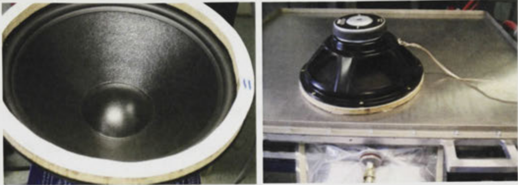
Figure 4.8: Subwoofer speaker (a) and in place on the top of the chamber (b).
