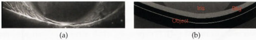
Figure 8.4: (a) Cropped image of the lower meniscus. (b) Object and background seed points. The furthest pixels from the initial spline can be ignored in the segmentation process.
