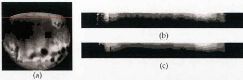
Figure 6.7: Example of an x - t cut. (a) Segmentation result using the new approach. An x - t cut (not to scale) at the location of the line in (a) using the (b) 2D approach. (c) 3D approach. The y -axis in (b) & (c) shows temporal progress from bottom to top.
