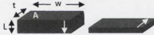
Figure 2.15: Geometry for defining sheet resistance. The measure of current flow is parallel to the length of the conductor, as shown by the white arrow.
