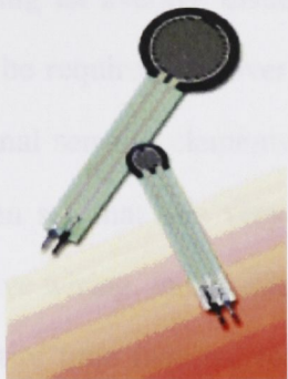
Figure 40: Interlink® FSR 400 and 402, Force Sensing Resistors.
