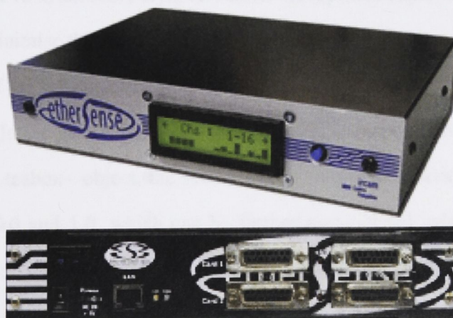
Figure 49: The EtherSense OSC/MIDI sensor interface.
