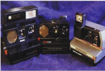
Figure 25: Various Polaroid® cameras that utilise an ultrasonic ranging device.
