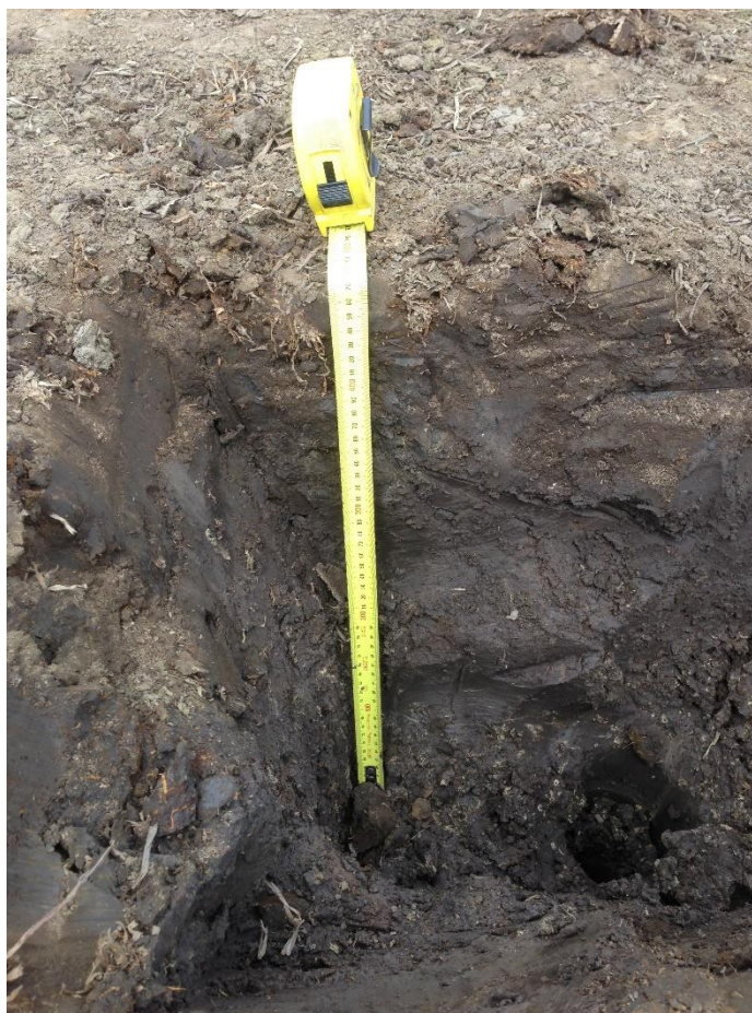
Plate 3.1 Acid sulphate soil with a jarosite layer 50 cm below soil surface
