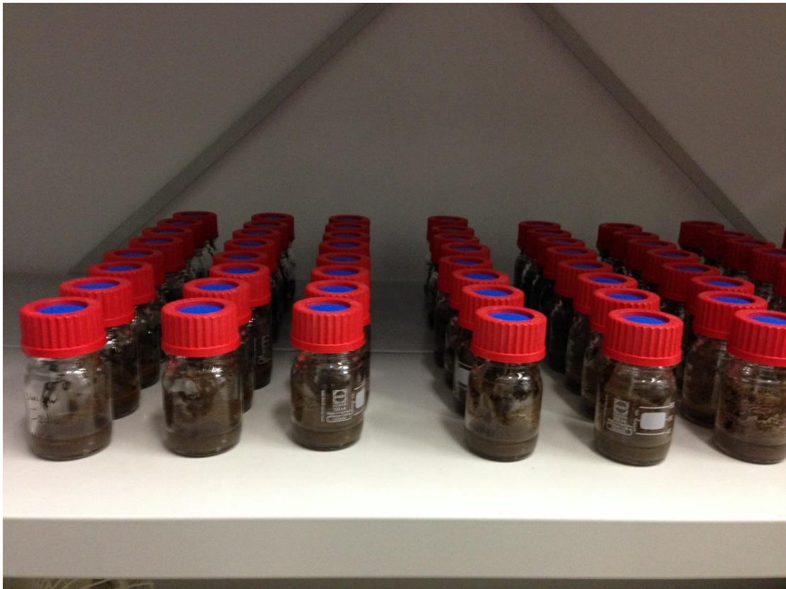
Plate 4.1 Soil with different salinity level was incubated in jars at constant temperature (25°C). The photo was taken before sampling headspace gas.
