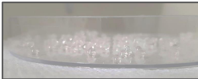
Figure 3:17: Lenses of various heights produced using the passive droplet approach. The high throughput of this moldless approach also has one added advantage, that the cost per lens does not depend on the number of lenses produced. The lenses cost ~1 cent per lens.
