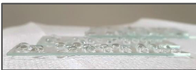
Figure 3:18: Plano-convex lenses of various diameter and heights manufactured using the simple active dispenser.
