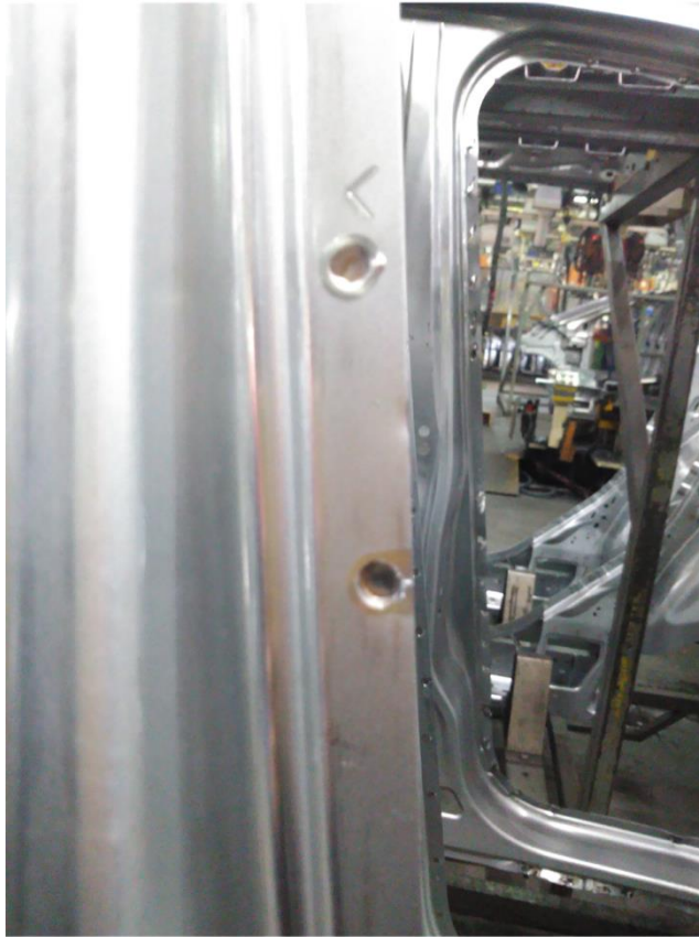
Figure 2.39 Spot welds close to edges in the B-pillar
