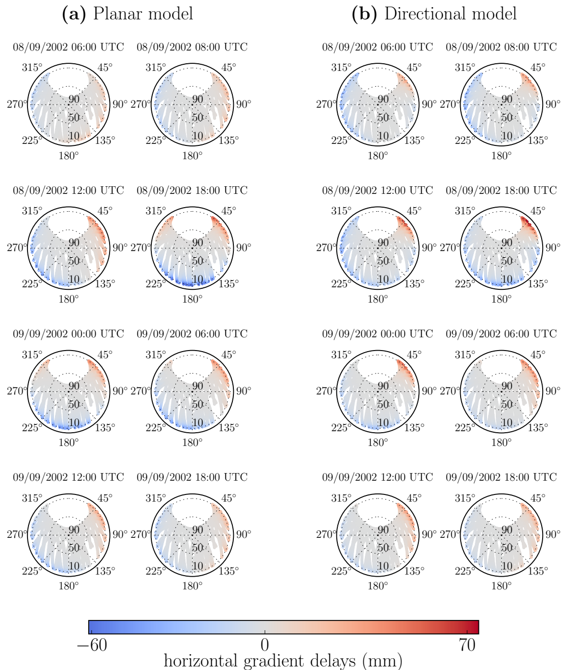
Figure 4.14: Horizontal gradient delays estimated at site MTPL using (a) the conventional planar model, and (b) the directional model with 8 gradient estimation nodes. The horizontal gradients are isolated towards the north-east by the directional model.
