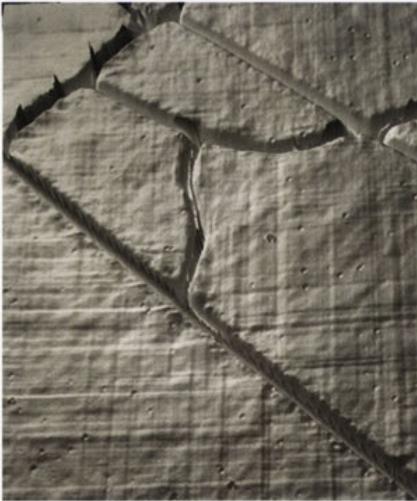
Figure 3.6: The optical profiler image of the dislocation network formed in the silicon substrate by the tensile stress in a \text{SiO}_{1.16}\text{N}_{0.32}\text{:H} layer after annealing at 1100^\circ\text{C} .
