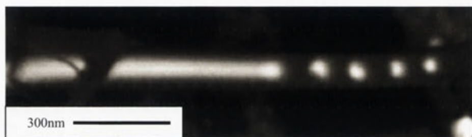
Figure 5.10: Au wire in silica nanowires grown by coating a silicon wafer with 10 nm of Au and annealing at 1100°C in N 2 for 1 hour with Si capping layer then re-annealing the sample under the same temperature and ambient but annealing time for 20min without its capping layer (The growth direction is towards the right and the wire is capped by Au head, which is not included in the image).
