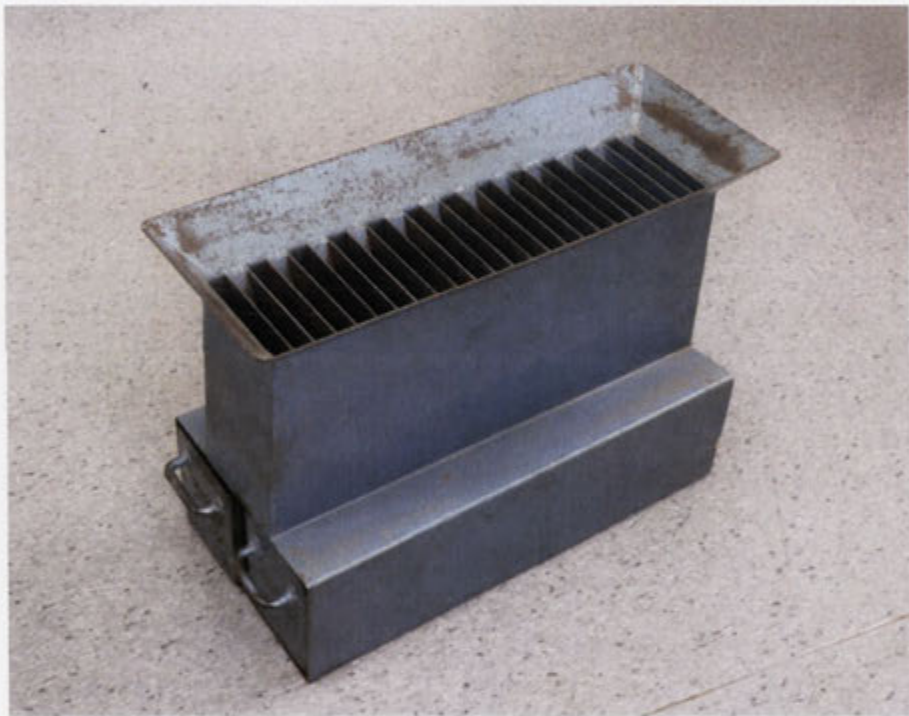
Figure 9.3 Geo-splitter used for sub-sampling of soil samples for analysis of seed abundance from floristic plots on Helen Springs Station.
