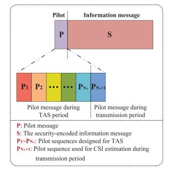
Fig. 1. The frame structure of TAS and secure transmission.
