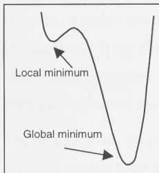
Figure 7 - Global and local minima for a hypothetical function. The temperature in a simulated annealing algorithm helps it to escape from local minima in the multi-dimensional solution space of the problem, represented here in simplified form.
