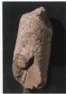
2 CBAC 85 (1-2m) Laminated mudstone with carbonate veinlet
