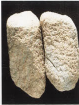
1 CBAC 40 (1-2 m) Sandy silty mudstone with carbonate veinlet
