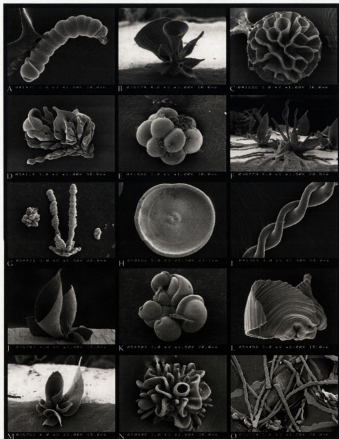
Figure 3.1: A taste of the different biomorph morphologies discussed in this chapter; worms (A), trumpets and cones (B, F, J), coral-like floral spherulites (C, N), globular (E, K), pinnacles (G), disks (H), double helices (I), sheets (F, L, M), bands (O). An aggregate displaying a mixture of different morphological traits (sheets, globules, pinnacles) can be seen in D.
