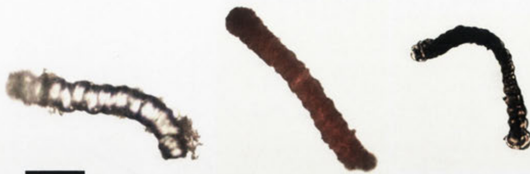
Figure 6.4: The color change of biomorphs seen during the condensation and curing of phenol formaldehyde. Left: as prepared biomorph. Middle: Biomorph after hydrothermal treatment with aqueous phenol and formaldehyde solution. Right: Structure after curing at 500 °C. Scale bar 50 \mu\text{m} applies to all three images.
