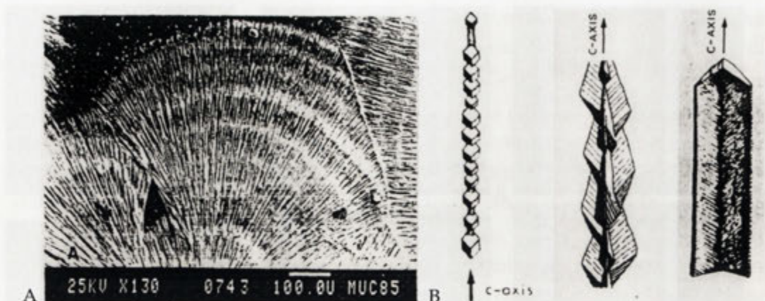
Figure 1.6: SEM image of a \text{CaCO}_3 biomorphs with banded sheaf of wheat morphology (A). Different kind of fibre design observed in banded (far left) and non-banded sheaf of wheat aggregates. Adapted from Dominguez Bella and García-Ruiz (1986).
