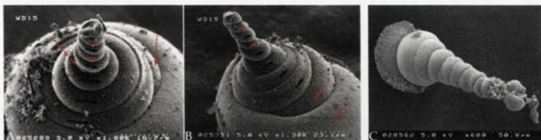
Figure 3.6: FESEM images of a helix-worm transition. The red arrows indicate one strand while the black arrows indicate the other. The red dashed arrows indicate the disappearance and resurfacing of the the red strand. In C an overgrown worm is seen with a characteristic head as well as large euhedral witherite crystals.
