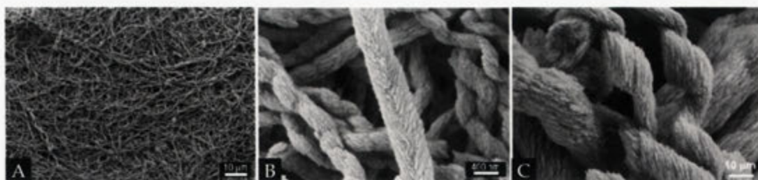
Figure 2.17: SEM images of \text{BaCO}_3 filaments grown in the presence of PEG- b DHPOBAEE, at an initial pH of 4. Adapted from Yu et al. (2004a).
