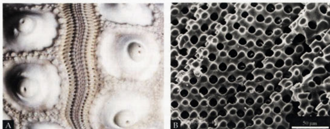
Figure 2.37: Detail of a sea urchin skeleton (test) in A, and SEM micrograph of the periodic calcitic structure. Image in A adapted from http://www.rsphysse.anu.edu.au/admin/php/images/photos/shell.jpg , Urdate 2006-09-18; B adapted from Yue et al. (2006).
