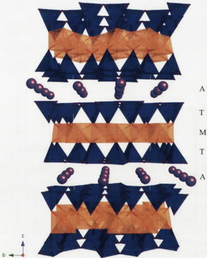
Figure D.2: The muscovite structure, where the blue tetrahedra represents (\text{Si, Al})\text{O}_4 tetrahedra (T) linked by orange octahedral cations (M). These layers are in turn sandwiched between large interlayer cations (A). Models were made with CrystalMaker, using crystallographic data from the CrystalMaker Library.
