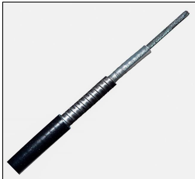
Figure 8: A standard Bowden cable design. From outer to inner: plastic sheath, metal coil, inner plastic tube, and actuating inner cable. The housing, metal coil, and plastic tube comprise the stationary housing.
