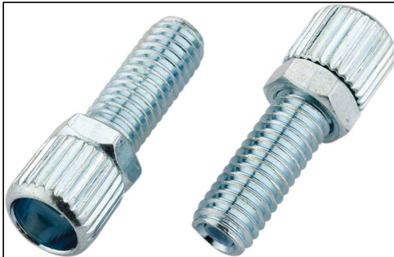
Figure 30: A barrel adjuster allows fine tuning of tension in a Bowden cable by controlling the distance between the end of the housing and the end of the cable.
