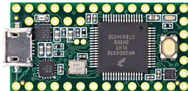
Figure 23: The Teensy 3.2 is an Arduino-based microcontroller with the necessary I/O connections and computing power to operate one joint.
