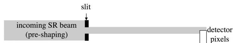
Figure 1. The basic implementation of the edge illumination method with synchrotron radiation.
